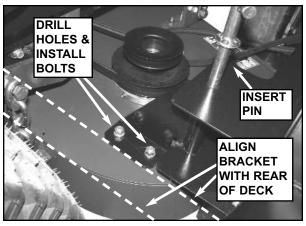
STEP 7: Slip tube of locking pin bracket into blower mount, and secure with T-handle pin, making sure pin goes through both upper and lower holes in blower mount. Then align base of pin bracket parallel with rear of deck, and, using bracket as a template, drill two 7/16" holes through deck. Insert two 3/8-16 x 1" hex bolts up through deck and bracket, securing with hex flange lock nuts. Tighten securely. IMPORTANT: Use gloves when working under deck. Sharp blades can cause injury.
